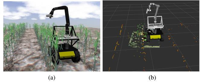
Figure 3: (a) Simulation of Vinobot in the field using Gazebo, and (b) Visualization of the real Vinobot and sensor data by Rviz. The orange points are parts of the plants detected by the LiDAR. The figure also displays the 3D point cloud being created by the stereo camera handled by the robotic arm.
