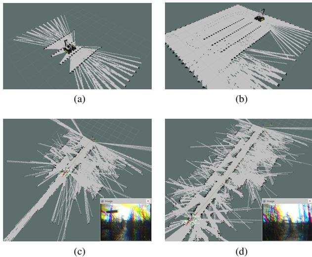
Figure 7: Visualization of Vinobot in Rviz while localizing itself and mapping the environments in (a, b) Gazebo simulation, and (c, d) real world using LiDAR, IMU, and GPS sensors.
