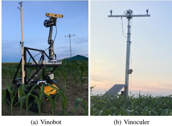
Figure 1: *The developed platforms for high-throughput phenotyping in the field deployed at the Bradford Research Facility: (a) ground vehicle, Vinobot; and (b) observation tower, Vinocular shown at the height of 15ft*
