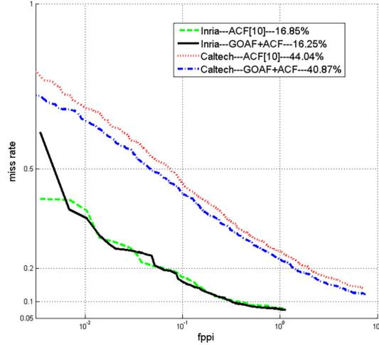
**Fig. 6.** Experimental results of GOAF with ACF on Caltech and Inria.
