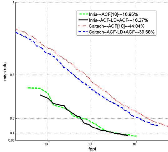
Fig. 7. Experimental results of ACF-LD with ACF on Caltech and Inria.
