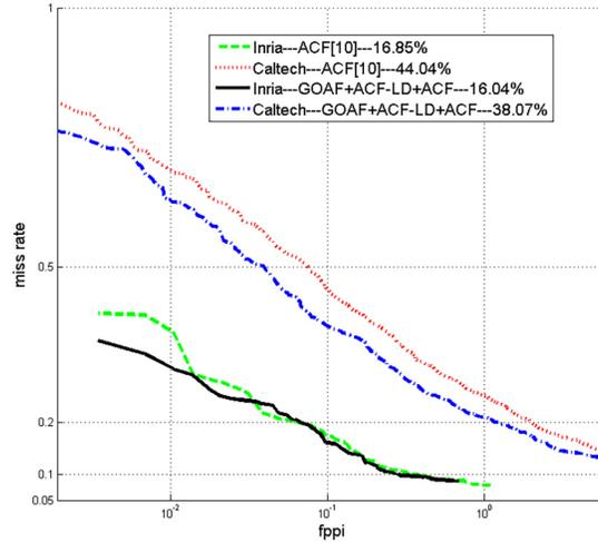
**Fig. 8.** Experimental results of GOAF, ACF-LF with ACF on Caltech and Inria.
