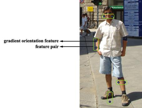
**Fig. 3.** The sample of different feature pairs for GOAF.
