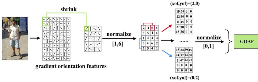
Fig. 4. The computing process of GOAF.
