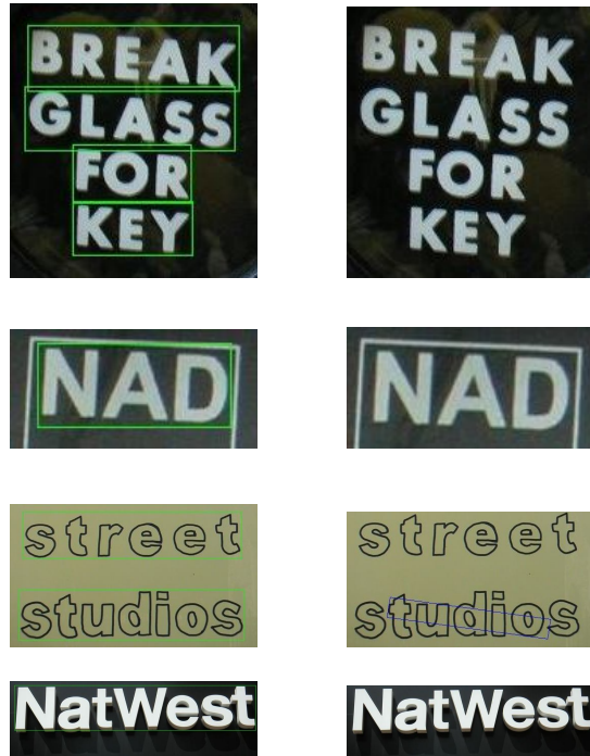
Fig. 1. Some texts in natural scenes which can be detected by the CC method ( left ) but not the sliding-window method ( right ). Rectangles indicate detected texts.
