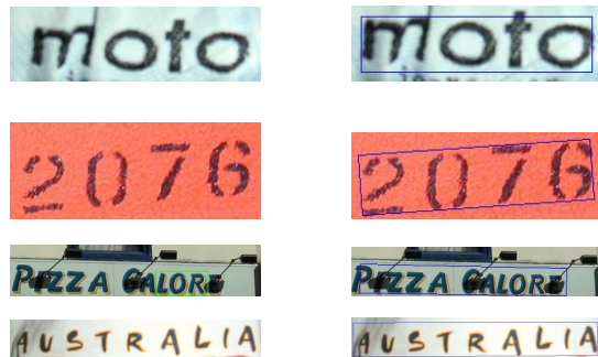
Fig. 2. Some texts in natural scenes which cannot be detected by the CC method ( left ) but can the sliding-window method ( right ). Rectangles indicate detected texts.
