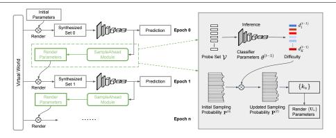
Figure 1: The overall framework of our approach. Without the SampleAhead module, our approach degenerates to that fixing a synthesized dataset at the very beginning and traversing all training samples orderly. Each SampleAhead module conducts an interactive process between the classifier and the sampler, in which the classification results in a standalone probe set are used to estimate the new training data distribution, from which the sampler generates the new set for the next training epoch.
