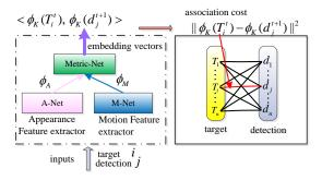
Figure 1: Architecture overview. In affinity model (dashed rectangle), the A-Net and M-Net extract appearance and motion cues, respectively. Both cues are combined in Metric-Net with a triplet loss function to produce the desired embedding features. For association (solid rectangle), a bipartite graph is constructed by association cost between already tracked targets and newly detections, and matching is achieved by Hungarian algorithm.
