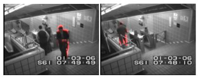
(a) True Positive (b) False Positive Figure 6: True positive and false positive detections on Subway dataset
