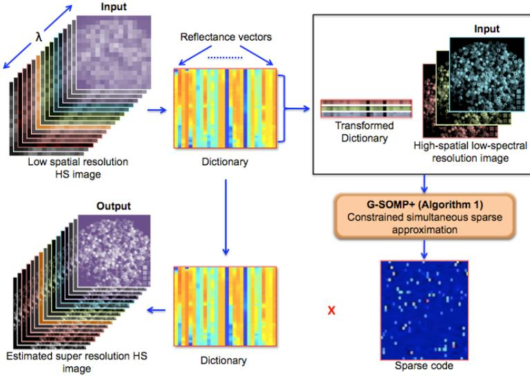
**Fig. 1.** Schematic of the proposed approach: The low spatial resolution hyperspectral (HS) image is used for learning a dictionary whose atoms represent reflectance spectra. This dictionary is transformed and used with the high-spatial but low-spectral resolution image to learn a sparse code by solving a constrained simultaneous sparse approximation problem. The sparse code is used with the original dictionary to estimate the super-resolution HS image.
