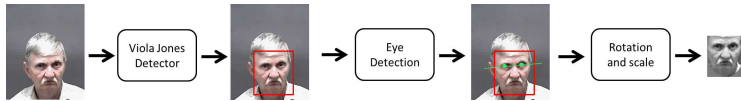
Fig. 3: The face detection and normalization step: the face is cropped and aligned in order to guarantee a standard pose to the features extraction step.
