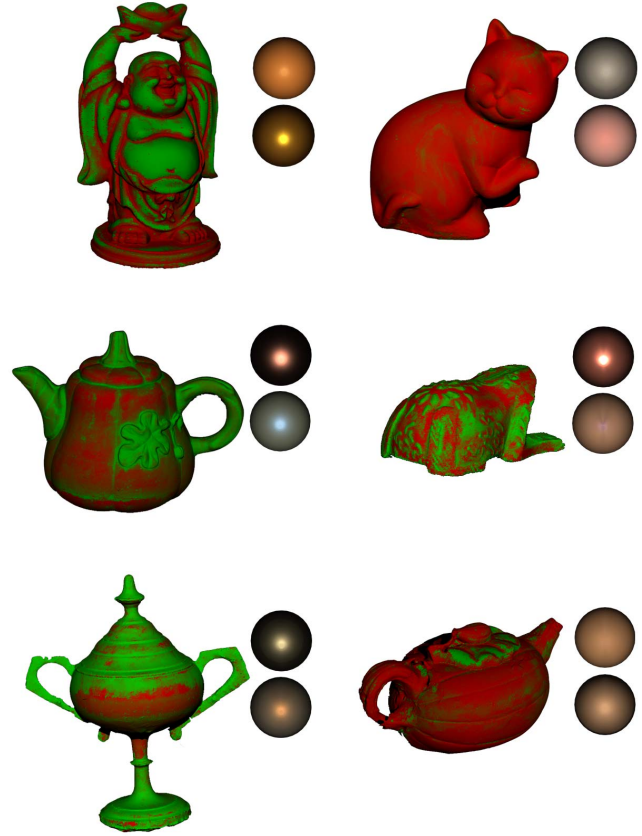
Figure 5. The normalized BRDF mixture weights are visualized in the different color channels. The corresponding basis BRDFs are used to render a sphere on the right.
