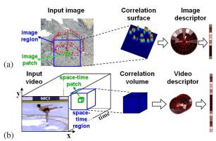
Figure 2. Extracting the local "self-similarity" descriptor. (a) at an image pixel. (b) at a video pixel.
