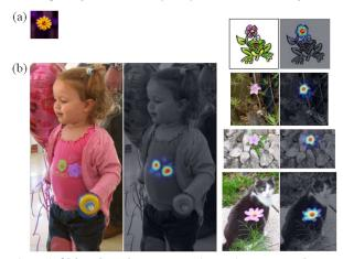
Figure 4. **Object detection.** (a) A single template image (a flower). (b) The images against which it was compared with the corresponding detections. The continuous likelihood values above a threshold (same threshold for all images) are shown superimposed on the gray-scale images, displaying detections of the template at correct locations (red corresponds to the highest values).
