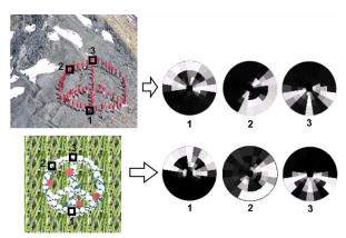
Figure 3. Corresponding "Self-similarity descriptors". We show a few corresponding points (1,2,3) across two images of the same object, with their "self-similarity" descriptors. Despite the large difference in photometric properties between the two images, their corresponding "self-similarity" descriptors are quite similar.
