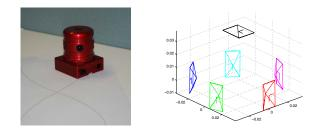
Figure 8. Left: our experiment setup. A ladybug camera is moving along a plotted planar curve; Right: spatial configurations of its six camera units.
