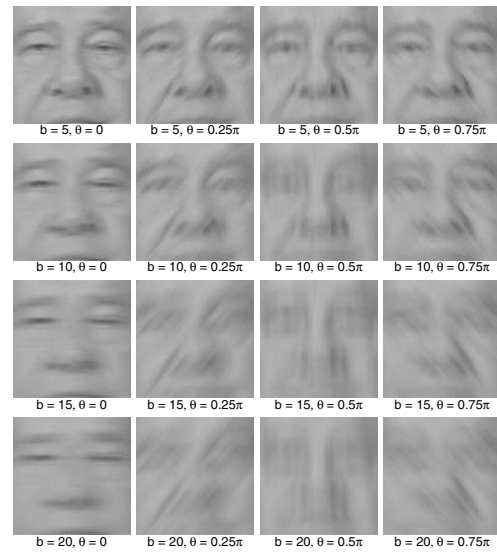
Figure 8. Examples of synthesized images of camera motion blur from the subset ‘fb’ of FERET. Blurred images are synthesized from Figure 5 (a) using linear motion blur PSFs with given b, \theta .
