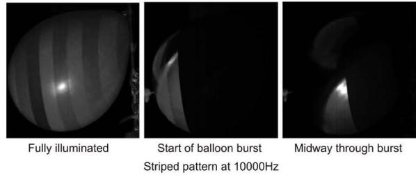
**Figure 9. DLP illumination as a programmable shutter:** On the left we show a balloon illuminated by a striped pattern from a DLP projector. Each stripe dithers at a different rate. We show two instances just after the balloon is burst, showing the edge of the contracting balloon in two different positions. If the pattern was uniformly set to either the first or second stripe value, one of these events would have been missed.
