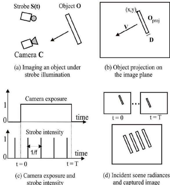
Figure 2. **Image formation model:** Consider a scene illuminated with a strobing light source, as in (a). Let an object move in a plane parallel to the image plane and at constant velocity, as in (b). Since the illumination is a dirac comb, the photograph can be modeled as a dot-product between a video of a moving object with the illumination, as in (c). The number of photographs is determined by the camera exposure, producing an image, (d).
