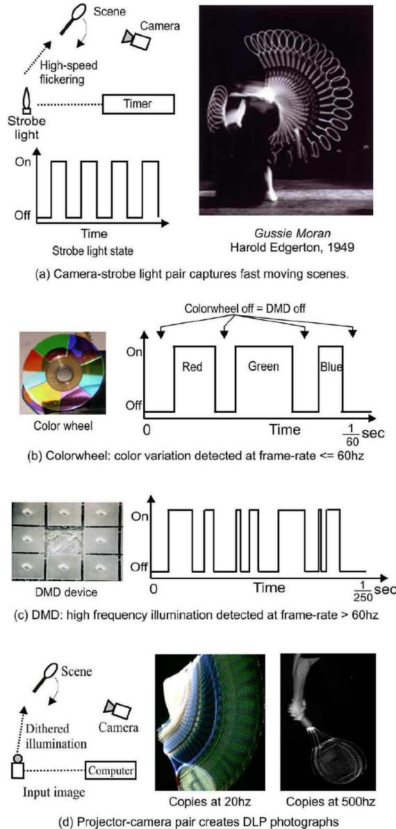
Figure 1. **Photographing fast moving scenes with varying illumination:** In (a) we show Edgerton's setup, which photographed moving scenes without motion blur using a strobe light. Strobe-light photography produces high-frequency object 'copies'. In (b) we show our setup with an unsynchronized DLP projector illuminating the scene. Both the projector's DMD and its color wheel produce a similar strobe-like effect which we term the DMD-colorwheel effect, as shown in (d).
