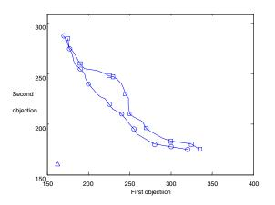
The point "box" in this chart is the point set on Pareto front is given by ST-GA; the point "lap" is the point set on Pareto front is given by Fuzzy-GA; "Triangle" is the ideal point. It is obviously that Fuzzy-GA method is superior to ST-GA in solving Pareto front.
