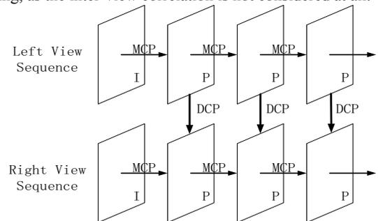
Fig. 1 Basic prediction structure of two-view based stereoscopic video coding
