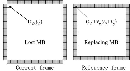
Fig. 4 Illustration of the block matching algorithm (BMA)
