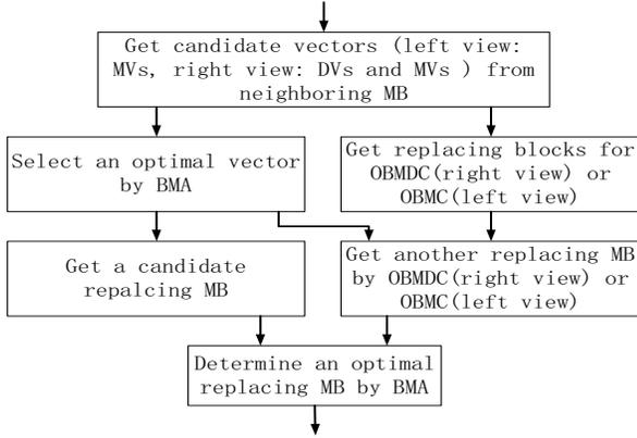
Fig. 2 Flowchart of the proposed error concealment algorithm with utilizing inter-view correlation and OBMDC
