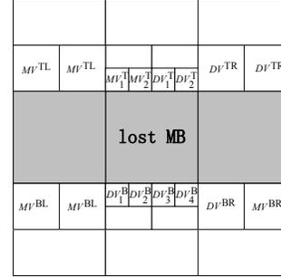
Fig. 3 Positions of the lost MB and the neighboring MBs with available motion or disparity vectors.
