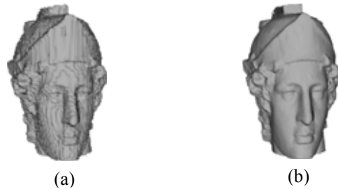
Fig.7 Rendering images of reconstructed models for “statue”. (a) TAGC scheme, coding rate: 5.31bpv, D_{rms} : 1.56, (b) PM-LWT scheme, coding rate: 5.05bpv, D_{rms} : 0.076.
