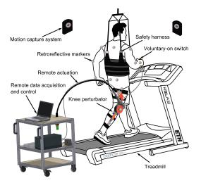
Fig. 1. Rendering of the proposed experimental environment for impedance estimation during level gait.
