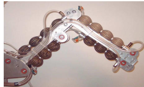
Fig. 1. The manipulator. The series arrangement of Pleated Pneumatic Artificial Muscles is clearly visible.
