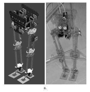
Fig. 1. (a) The 3D cad assembly of the robot. (b) The prototype, here with only one leg actuated.
