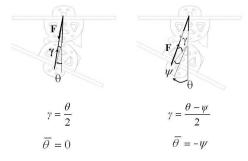
Fig. 3. We can exploit the action of the springs to impose a suited torque on the joint. In particular, it is possible to generate a position of instable equilibrium  $(\theta = \overline{\theta})$  to favor knee bending and stretching.
