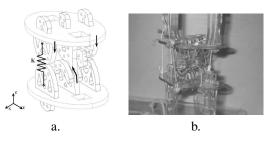
Fig. 2. (a) The knee joint designed for our robot. The arrows show the way the tendons are wrapped. (b) The knee prototype
