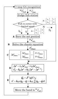
Fig. 2. Intelligent motion control process
