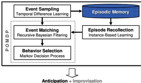
Figure 1: Computational steps for the anticipatory robot control
