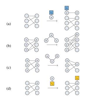
Fig. 6. Incrementally computing I-states in  $\mathcal{I}_{bip}$ : a) An appearance component event adds two vertices and an edge, with  $v_a$  associated with the left vertex. b) A split event splits a vertex and all edges pointing to that vertex. c) A merge event collapses two vertices into one and collapses their ingoing edges. d) A disappear event only associates  $v_a$  with the vertex on the right side.
