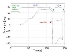
Fig. 5. The pan angle as a function of time. The camera behaviour alternates between tracking and exploration.
