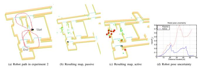
Fig. 6. Experiment 2: comparison of passive and active camera control. Green, small dots are landmarks (b,c), red, large dots are database matches (c). (d): the robot pose uncertainty computed as the trace of  $P_{rr}$  (covariance of robot pose) for passive and active camera mode. A video showing the trajectory of the robot in active camera mode is available on the CD proceedings of ICRA 2008.
