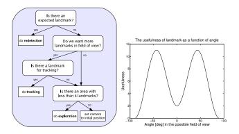
Fig. 4. Left: The three camera behaviours *Redetection*, *Tracking*, *Exploration*. Right: The usefulness function  $\varphi(\alpha)$ .
