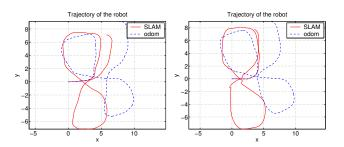
Fig. 7. Trajectory of robot path estimated from odometry (blue, dashed) and SLAM (red, solid) for passive (left) and active (right) camera mode.
