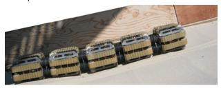
**Figure 2:** Our earlier-developed and larger OmniTread OT-8 can fit through an 8-inch diameter hole. Here it is driving up an inclined sand pit.
