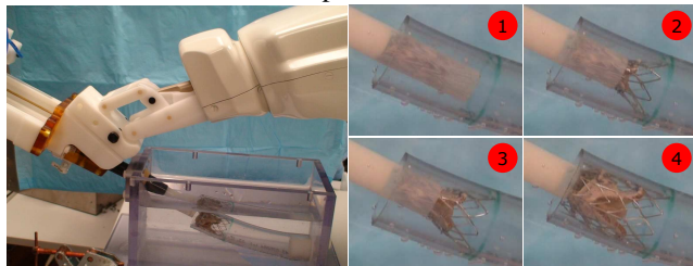
Fig. 5. (a) Experimental setup to test delivery module (b) Sequence of images showing the deployment of self-expanding prosthesis
