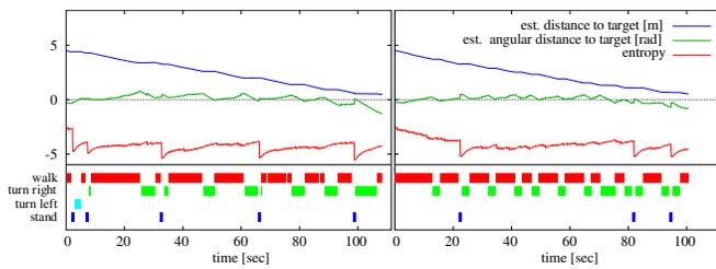
Fig. 6. The state features over time during typical runs with a hand-optimized controller (left) and the learned navigation policy (right) in simulation. The hand-optimized controller stops the robot in regular intervals to decrease the uncertainty, whereas the learned policy adapts the observation frequency according to the current state.
