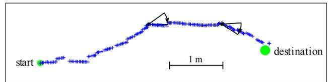
Fig. 5. Estimated trajectory of the Nao executing the learned navigation policy in our hallway. The robot walks forward with an error resulting from a drift to the left. Whenever it seems appropriate according to its belief, the robot executes a rotation action to re-align with the goal. The robot stops as soon as it recognizes the goal landmark.
