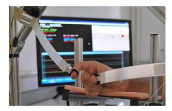
Fig. 1. *ReGrasp*, a robotic tool for precision grasp studies involving opposition of the index finger against the thumb in conjunction with functional brain imaging.
