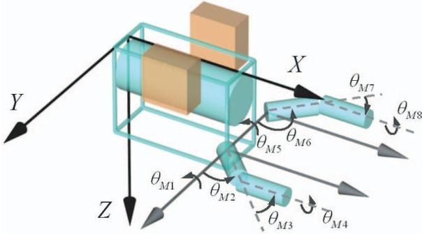
Fig. 8. Joint variables of manipulators
