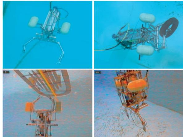
Fig. 1. Top left: A small UVMS "CoCo dexterity" with an attitude control system we developed. Top right: Removal of an old tire from a diving pool (demonstration). Bottom left: inspection of the bottom of a boat while the UVMS is facing upward (demonstration). Bottom right: UVMS is facing downward.
