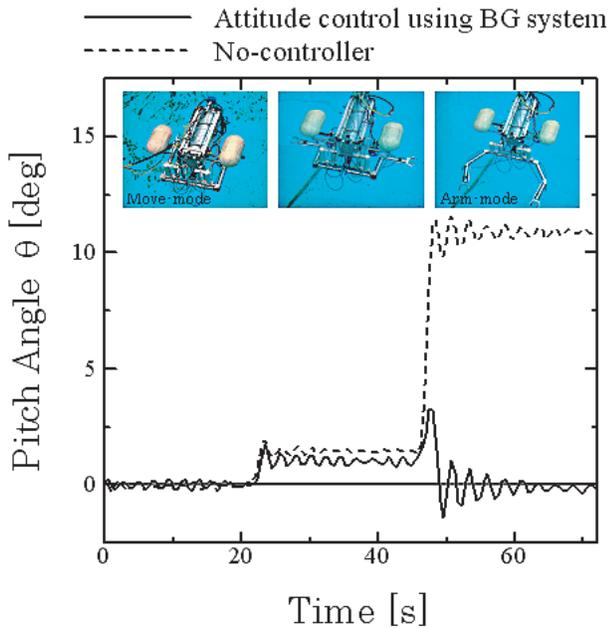
Fig. 12. Attitude-keeping control of BG system
