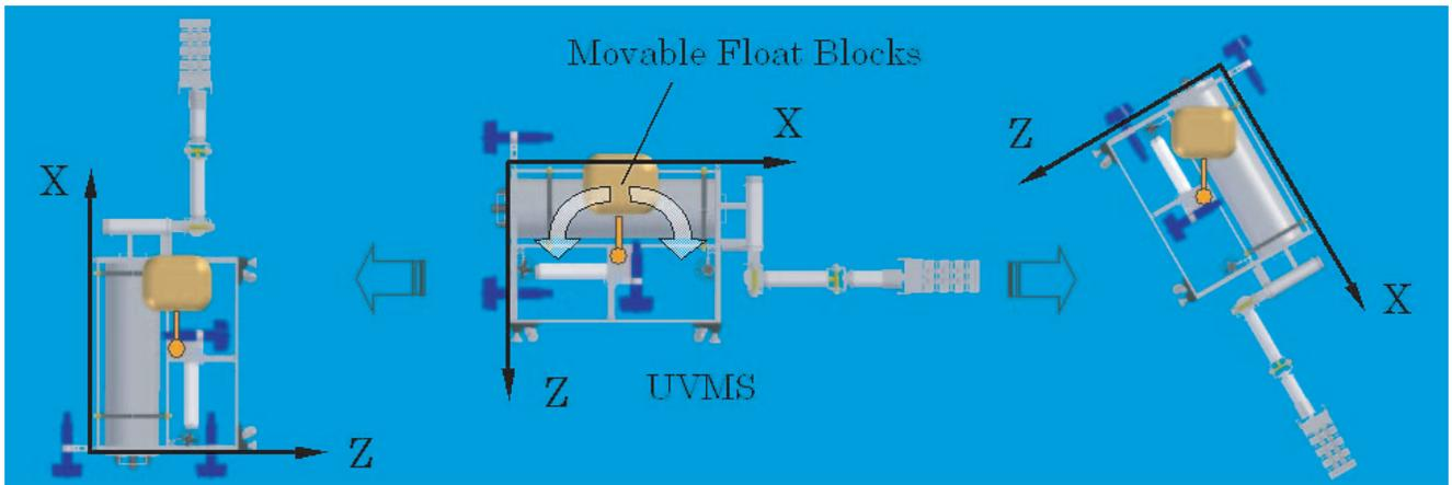
Fig. 2. Attitude Control System (BG system)
