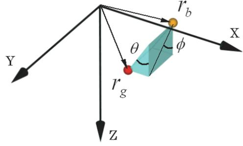
Fig. 5. Position vectors  $r_g$  and  $r_b$  used for attitude control
