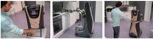
Fig. 9. The 'two sides' concept: The robot is commanded via the touchscreen to fetch a drink and serve it to the user. During the interaction, the working side of the robot with its arm points away from the user.
