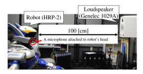
Fig. 8. Set up for impulse response measurement
