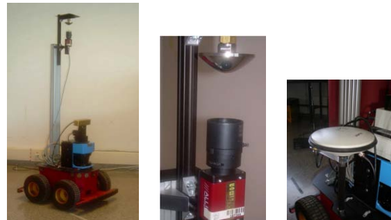
Fig. 1. Robot and sensors used, omnidirectional camera and GPS receiver.
