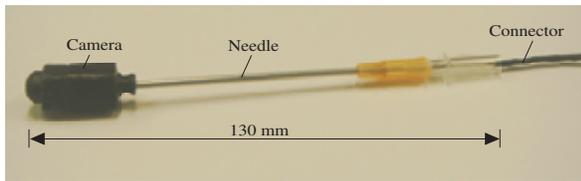
Fig. 2. An overview of the developed camera unit
