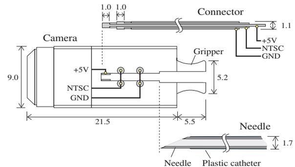
Fig. 5. Configurations of the camera unit
