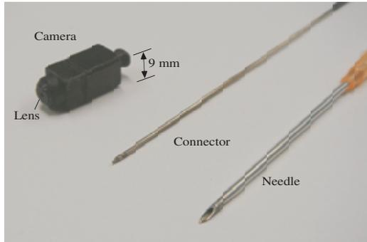
Fig. 3. The 3 parts of the camera unit
