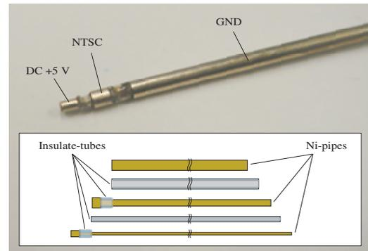
Fig. 4. Specifications of the connector
