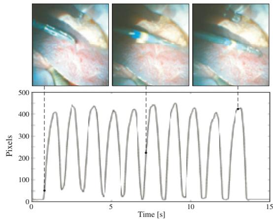
Fig. 11. An example of the detection of movement of the forceps determined from images obtained with the newly developed system
