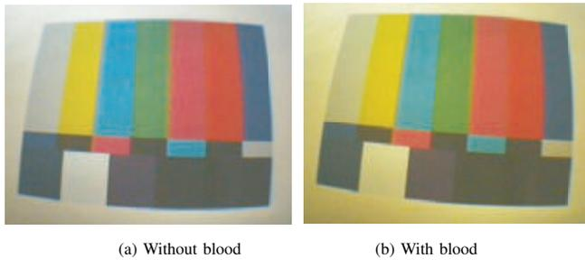
Fig. 13. Image noise by the attached blood to the connector part
