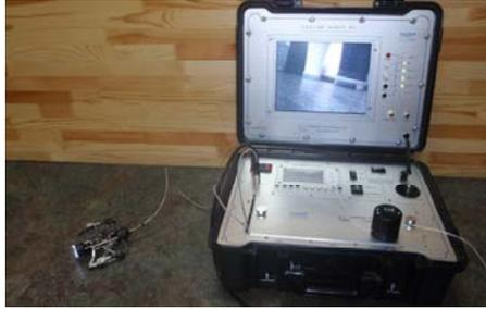
Fig. 1. The pipeline inspection robot system with a mechanical clutch.
