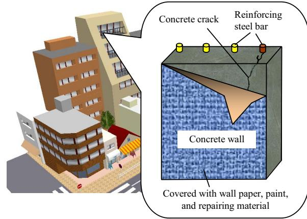
Figure 1. Deterioration of concrete structures by cracks
