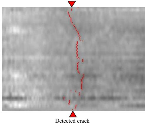
Figure 8. Result of image processing
