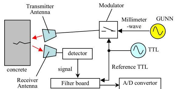
Figure 3. Configuration of active millimeter-wave imaging
