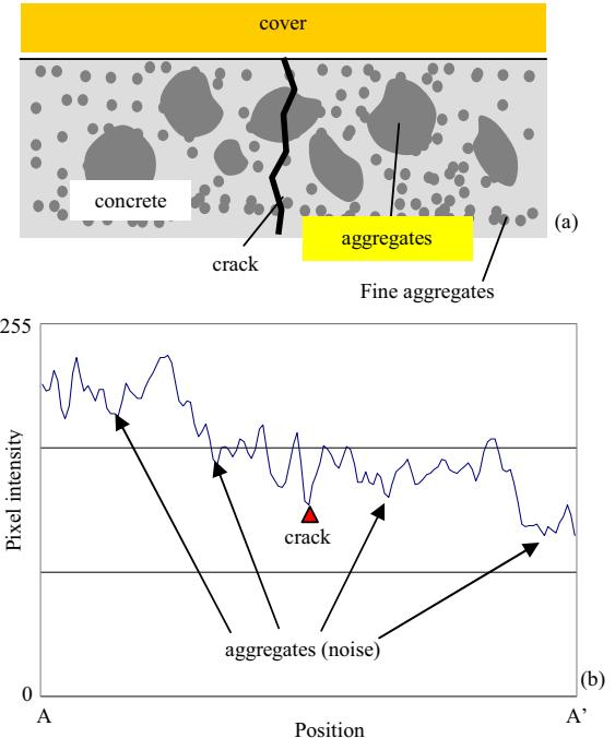
Figure 6. Invisibility of crack in millimeter-wave image. (a): Compositional non-uniformity of concrete, (b): Pixel intensity
