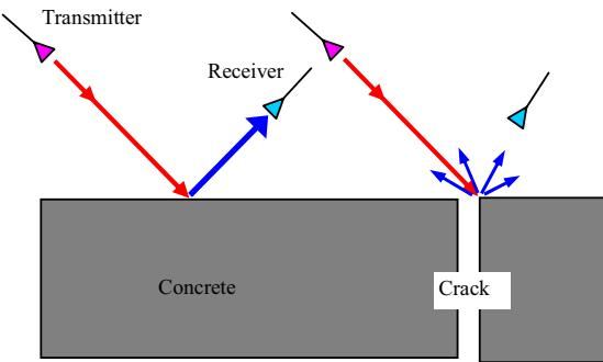
Figure 2. Surface reflection on concrete
