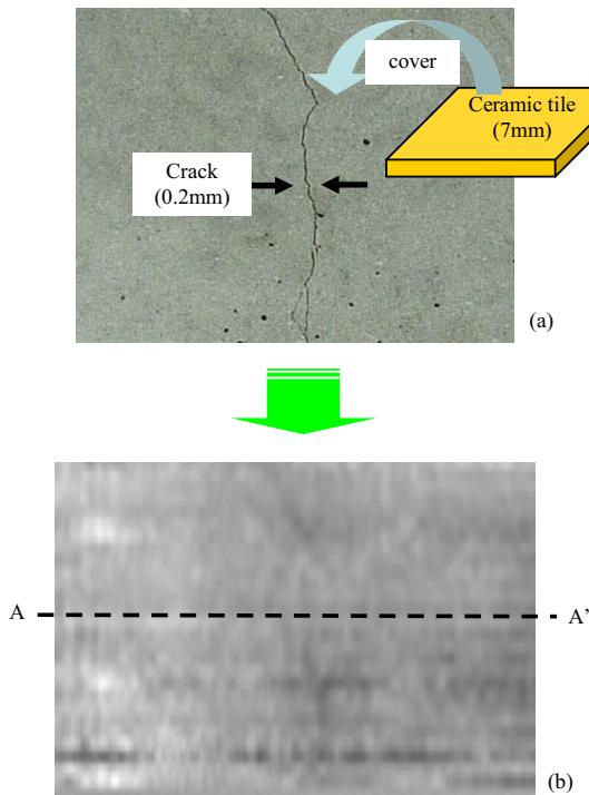
Figure 5. Millimeter-wave imaging of concrete surface crack. (a): CCD image of sample, (b): Millimeter-wave image (95 x 70 mm)
