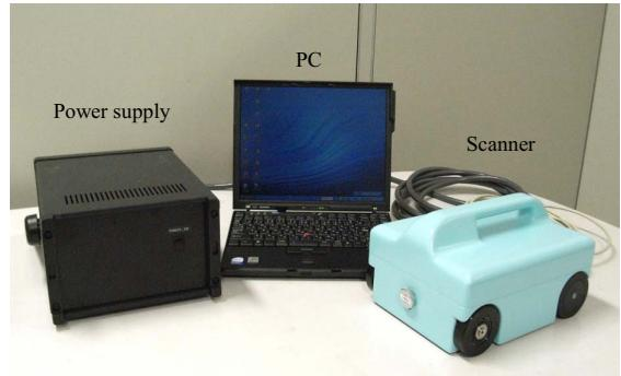
Figure 4. System design of Crack Scan
