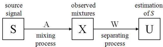
Figure 1. Blind source separation model.
