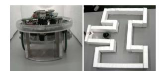
Fig. 1. Left: The e-puck robot developed at EPFL, Switzerland (http://www.epuck.org/). Right: The double T-maze environment including the light bulb and the robot.
