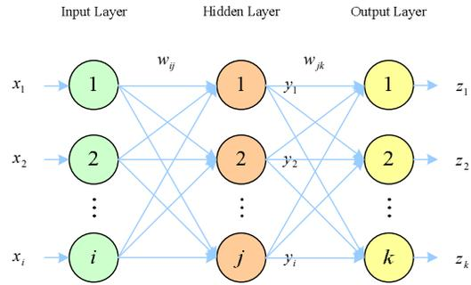
Fig. 2. The Structure of Back-Propagation Neural Network
