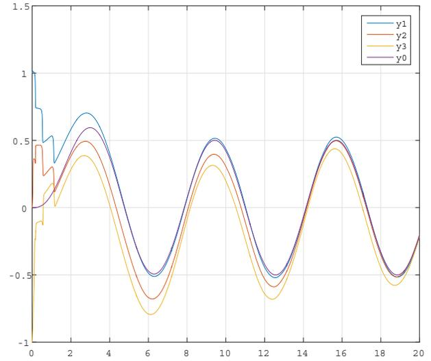
Fig. 5. Simulation Result for Time-Varying Case without  $H_\infty$  Control Scheme
