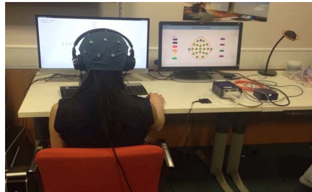
Figure 1: A photograph representing the experimental environment. The subject is placed by 80cm from the experiment's screen (on the left side). The second (on the left side) screen was used to continuously monitor the electrodes signal quality.
