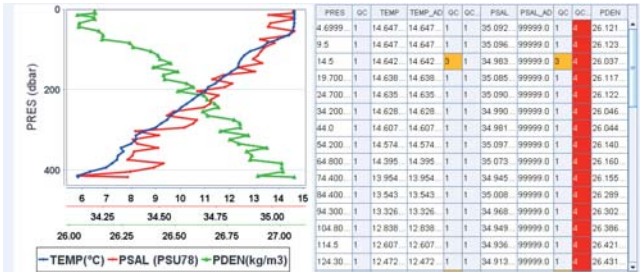
Figure 6. Example error over the whole profile (zigzag).
