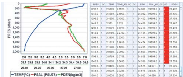
Figure 8. Example error over the whole profile (external factor).
