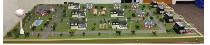
Fig. 2. RTPIS Lab Demand Response Research Platform
