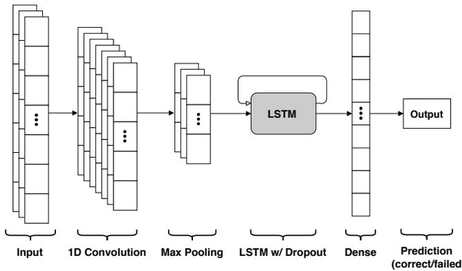
Fig. 3. LSTM network architecture: the input layer is followed by a 1D convolution layer (with 100 filters of size 20 and ReLU activation function), max pooling operation (with a pool size of 2), LSTM block (with 100 cells), dropout layer (with rate 0.5) and finally a dense layer with the sigmoid activation function.
