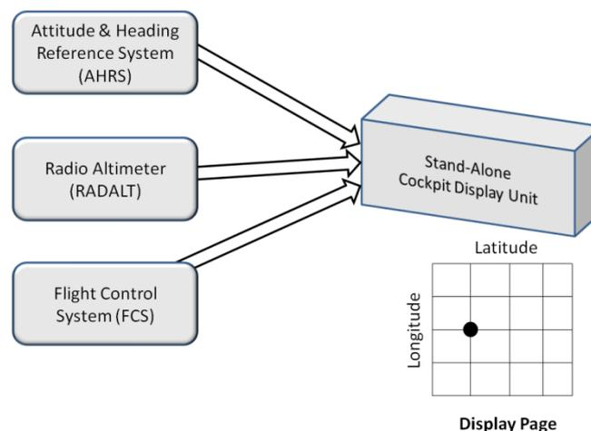
Fig. 1. Block Diagram of proposed Stand-alone Navigation System
