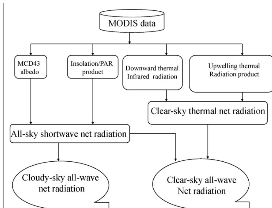
Figure 1 . Flowchart of the estimation of net radiation from MODIS
