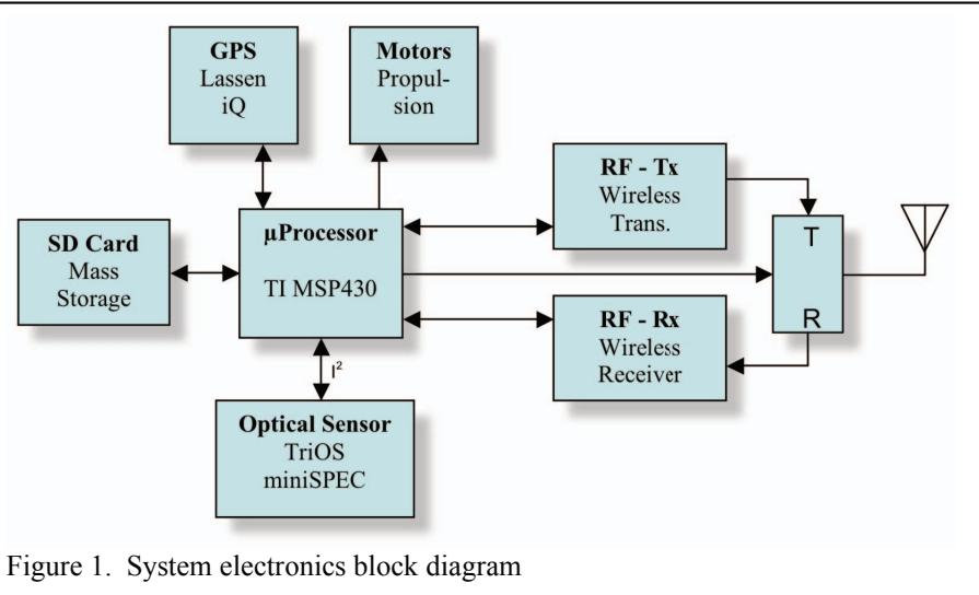
Figure 1. System electronics block diagram
