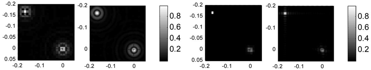
Figure 1: Images for two point targets. (a) BP, (b) upsample (a) by a factor of 7, (c) CS with  $J=100$ , (d) upsample (c) by a factor of 7.
