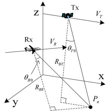
Fig. 1 GPS signal based SS-BSAR geometry
