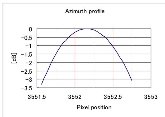
Fig. 4 Up-sampled range profile (left) and azimuth profile (right) of a CR (50cm-square). Pixel spacing is 0.25m x 0.25m.
