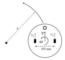
where  $\omega$ , v are angular and linear (forward) velocities, respectively. r is the radius of turning which can be found by r = v/w.
